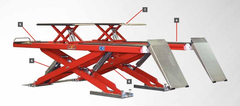
**4. Adjustable mechanical safety device**, also for exact adjustment for wheel alignment.
