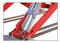
7. Lift table with double lifting cylinder and double extensions, in front and rear, which is very flexible, no movement of vehicle on the lift needed.
